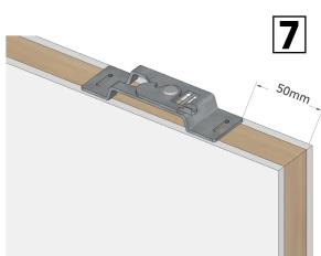
Fix both base plate 50mm to the edge of the door.
