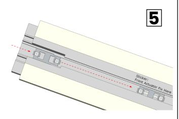
Loose the screws on the actuator. Insert actuator from the cut out and slide to cover the silver sticker. Tighten the screws to fix the actuator's position.
