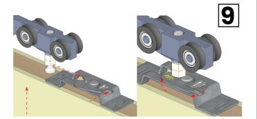
Lift the door to when the waist of the roller screw is facing the pening of the back plate.
