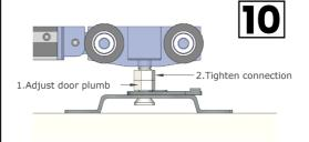
Use spanner provided to adjust the bottom nut on the roller screw, until the door is at the desired height and is plumb with the jamb.
